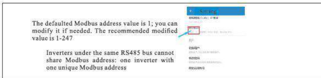
Figure 5.28 Modifying and saving Modbus address
