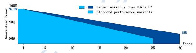
(4)For Monocrystalline double glass modules: not exceed 2.5% degradation in the first year, and 0.5% per year thereafter, ending at 83% in the 30th year after warranty start.
