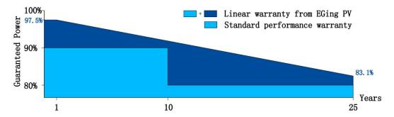
(3)For Polycrystalline double glass modules: not exceed 2.5% degradation in the first year, and 0.5 % per year thereafter, ending at 83% in the 30th year after warranty start.
